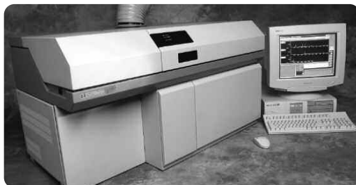
HP 4500 - the first benchtop ICP-MS. Hewlett-Packard Analytical Instruments Division formed part of Agilent Technologies in 1999.
