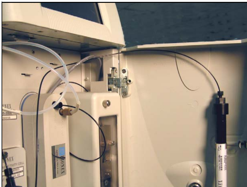
Figure B-75. Mixer Outlet Routed to the Back of the Component Panel
