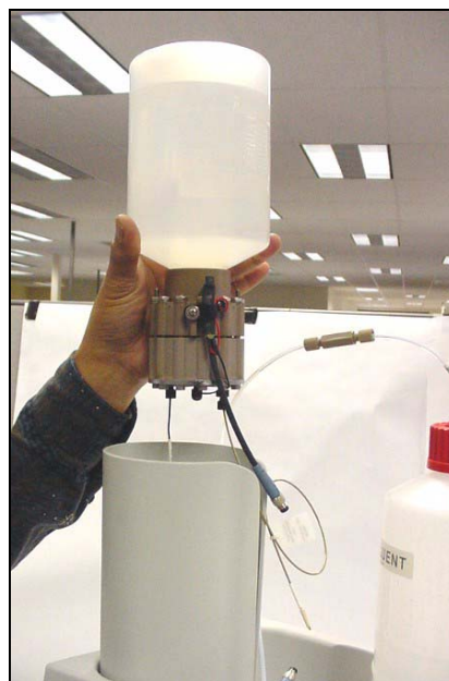
Figure 5-38. Installing the EluGen Cartridge in the Holder
