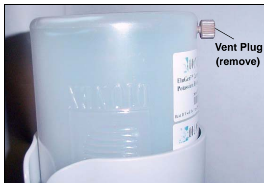
Figure B-59. EluGen Cartridge Vent Plug
