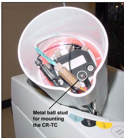
Figure B-32. Cartridge Holder (tilted to view the bottom)
