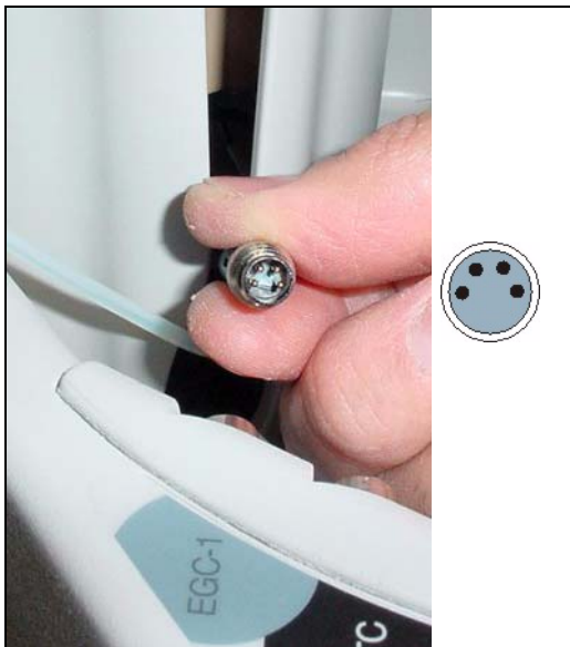
Figure B-82. Connecting the EluGen Cartridge Cable
