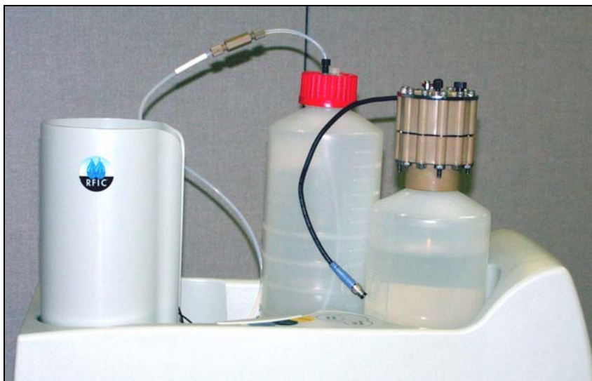
Figure B-38. EluGen Cartridge in Service Area
