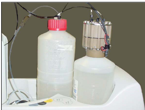
Figure 5-69. EluGen Cartridge in Service Area
