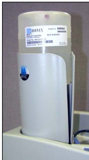
Figure 5-48. EluGen Cartridge Installed in the Holder
