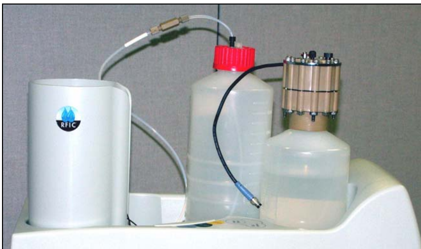
Figure B-79. EluGen Cartridge in Service Area
