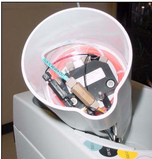
Figure B-51. Cartridge Holder (tilted to view the bottom)
