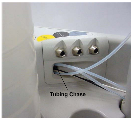
Figure 5-70. Top Cover Tubing Chase
