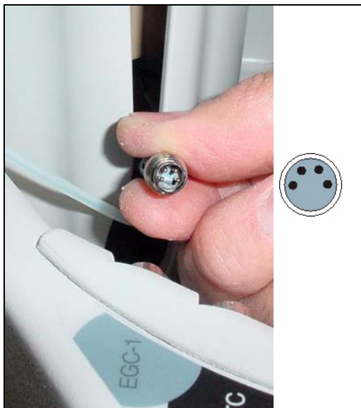
Figure 5-49. Connecting the EluGen Cartridge Cable
