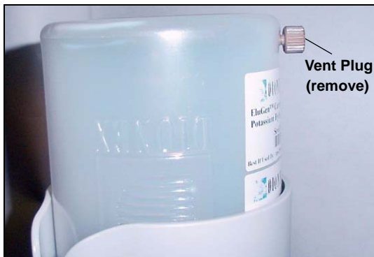
Figure B-84. EluGen Cartridge Vent Plug
