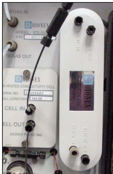
Figure B-23. Suppressor Installed (SRS Shown)
