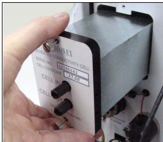
Figure 5-17. Removing the Cell Assembly
