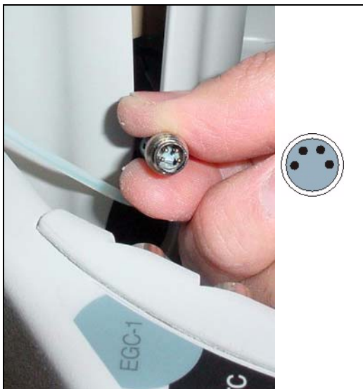
Figure 5-39. Connecting the EluGen Cartridge Cable
