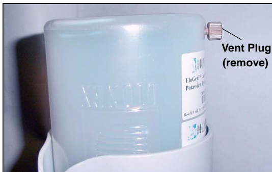
Figure B-43. EluGen Cartridge Vent Plug
