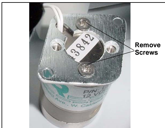
Figure 5-26. Removing the Valve Mounting Plate
