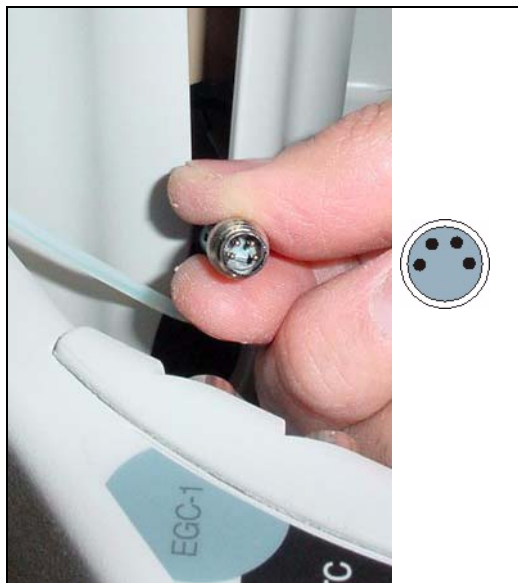
Figure B-58. Connecting the EluGen Cartridge Cable
